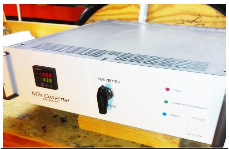
Molybdenum based converter Operating temperature > 316C Flowrate > 2lpm
